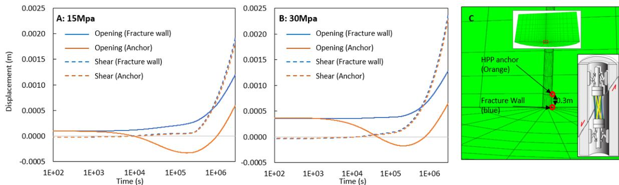
**Figure 1. Wellbore response of fracture wall and HPP anchor. Blue denotes fracture wall, orange denotes HPP tool response, solid line denotes fault opening displacement and dashed line denotes fault shear displacement.**
