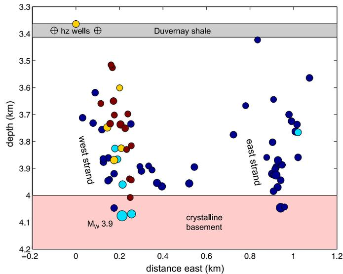
**Figure 1:** Cross-section through a cluster of induced seismicity, showing east and west fault strands inferred from double-difference event locations (Bao and Eaton, 2016). Dark blue symbols show events that occurred during hydraulic fracturing in two horizontal (hz) wells. Light blue, yellow and red symbols show events during subsequent sequences.
