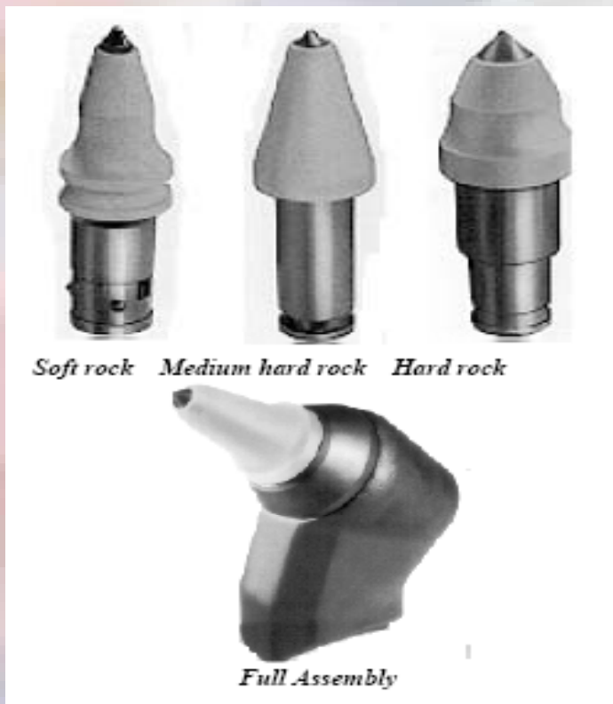
Figure 1. Various types of conical cutters and the forces acting on the cutters.
