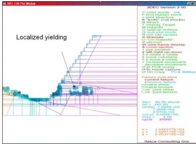
Figure 18. Vertical section through 3DEC model that is the same as the section shown in Figure 16. Only minor rock-mass failure is indicated in the three-dimensional model (FS > 1.50 )
