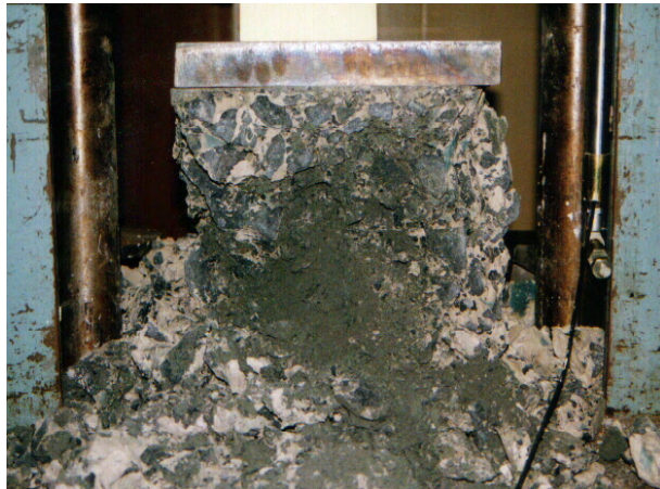
Figure 4 Large-scale laboratory unconfined compressive strength test.
